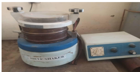
Fig. 2. Set up for abrasion resistance index determination
