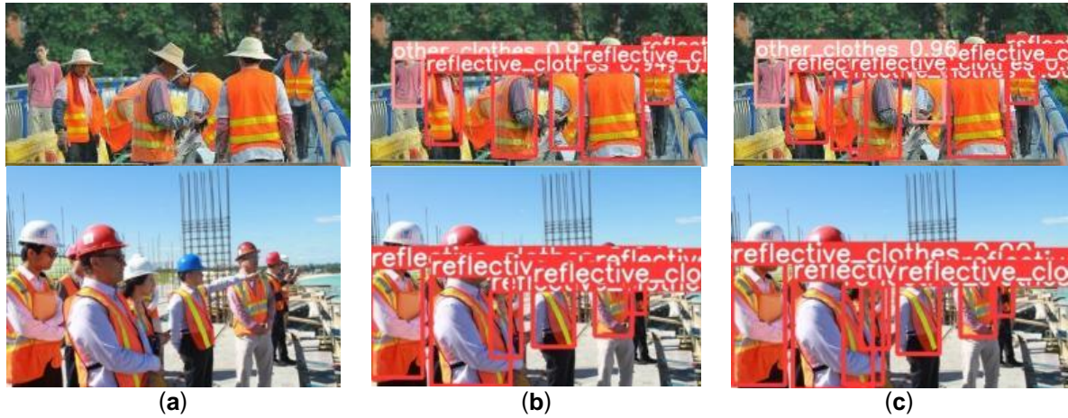
Fig. 12. Comparison of optimization effects of loss functions: (a) The original image; (b) Detection results based on YOLOv3; (c) Detection results of YOLOv3 with DIUO-NMS
