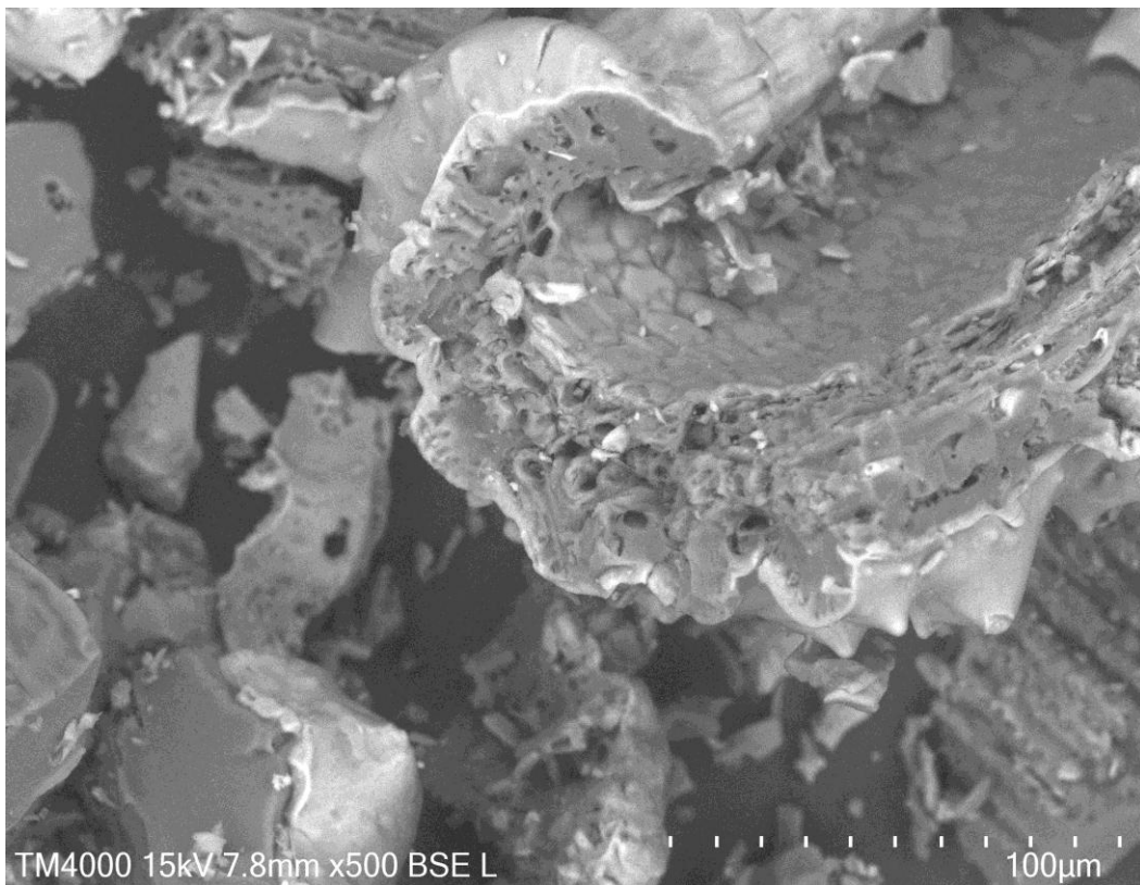
Fig. 3e. SEM micrograph of activated carbon after adsorption of paracetamol
