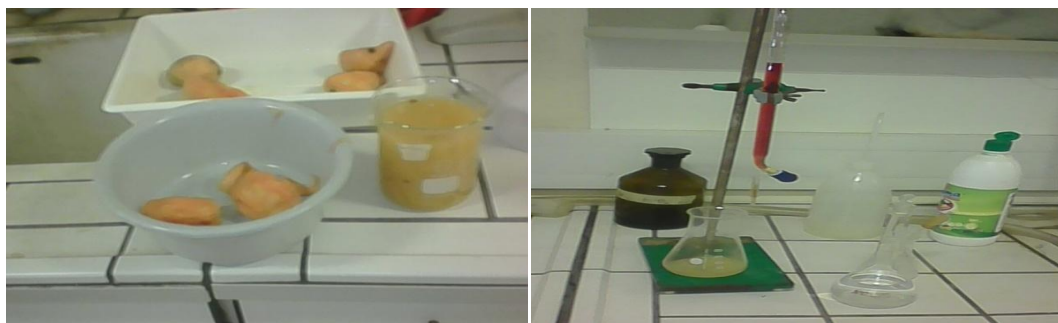
Fig. 4. Showing the blended mango juice and their titration with I_3^-
