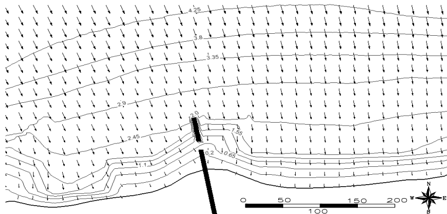
Fig. 9-b. Computed radiation stress (m/sec) during the occurrence of maximum incident deep water wave height in the vicinity of the groin ( H_i=4.6\text{m} , L_g= 100\text{m} , P=0.0 and S/ L_g=0.05 )
