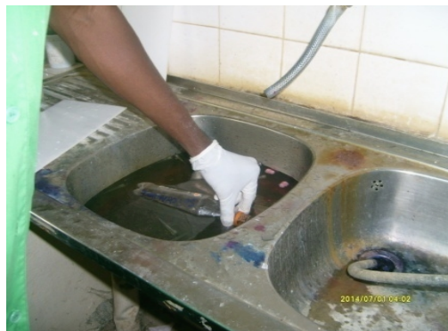
Fig. 6. collection of laboratory effluents samples from the sink with a plastic jar
