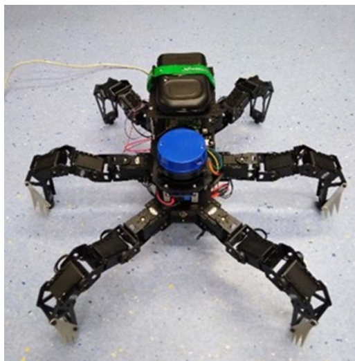
Figure 3. Photographic image of the off-the-shelf Phantom AX metal Hexapod MK-III by Interbotix lads. In this image a LIDAR and radiation detector are integrated to the robot.
