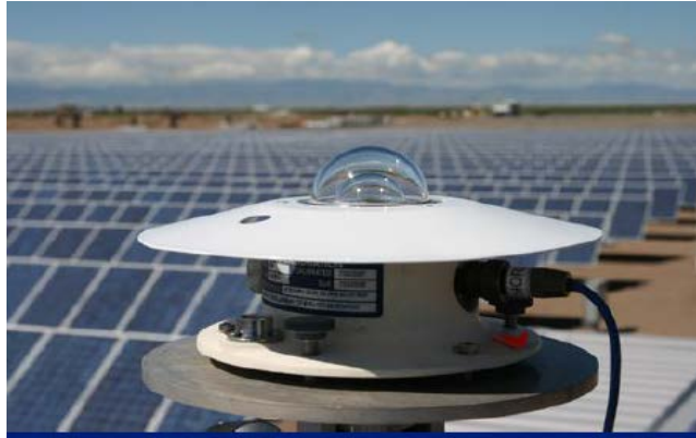
Figure 1. Pyranometer to measure the global solar radiation on the ground (GHI).
