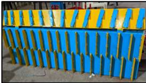
Fig. 6. Blade arrangement on developed clod crusher
