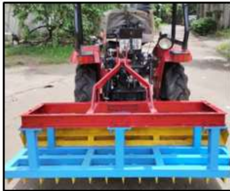
Fig. 5. Fabricated mini tractor-operated clod crusher
