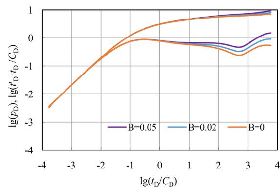
**Figure 2.** Effect of starting pressure gradient on pressure curve.
