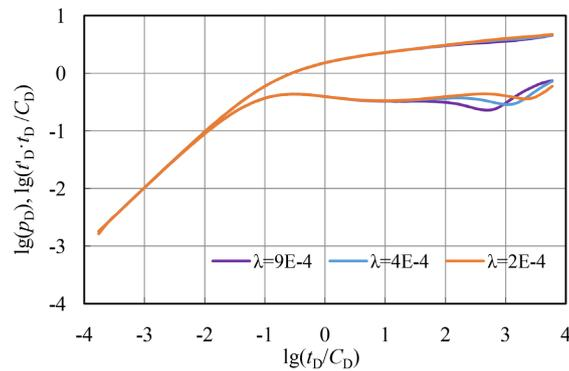
**Figure 3.** Effect of crossflow coefficient on pressure curve.
