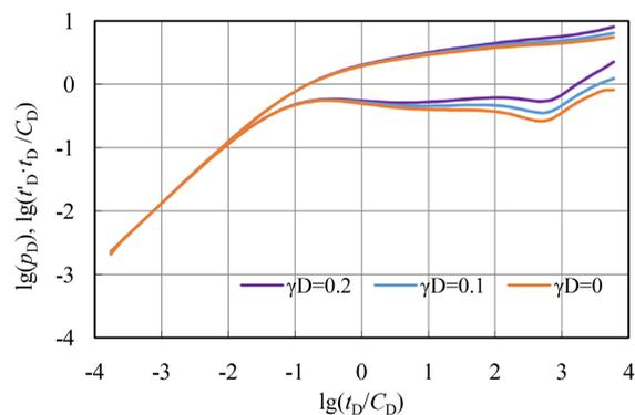
**Figure 1.** Effect of medium deformation on pressure curve.
