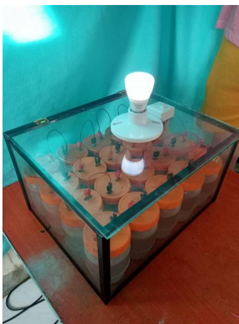
Fig. 21. Actual setup of a functional electrolytic cell with load
