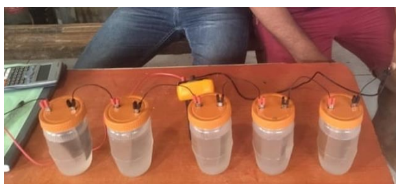
Fig. 16. Actual setup of cells in series connection
