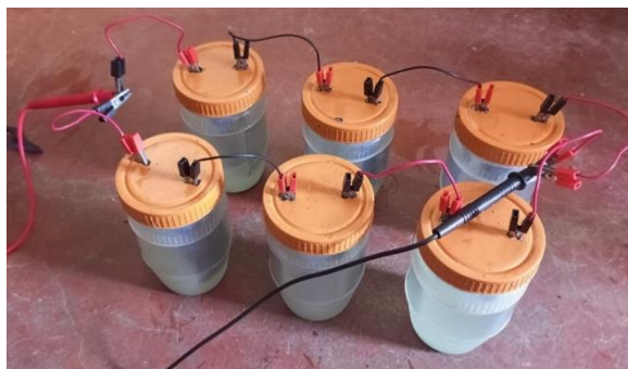
Fig. 19. Actual setup of cell in parallel-series connection
