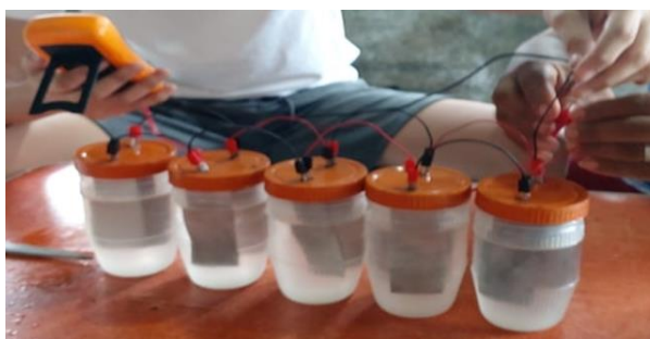
Fig. 17. Actual setup of cell in parallel connection
