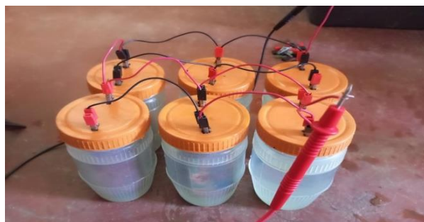
Fig. 18 Actual setup of cell in series-parallel connection
