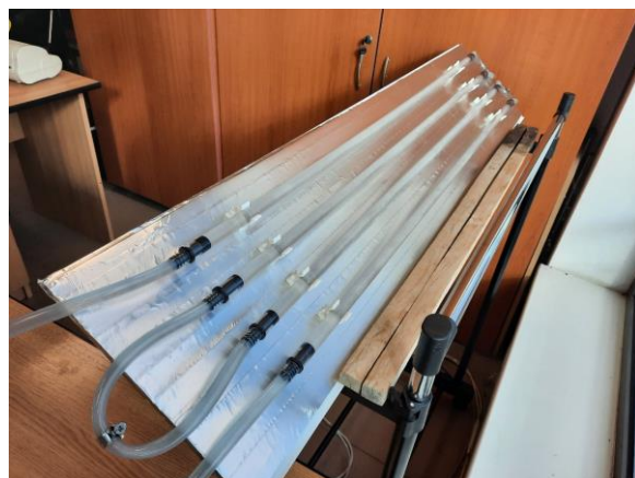
Figure 1. Solar photocatalytic installation used for PMR slurry photocatalytic step.
