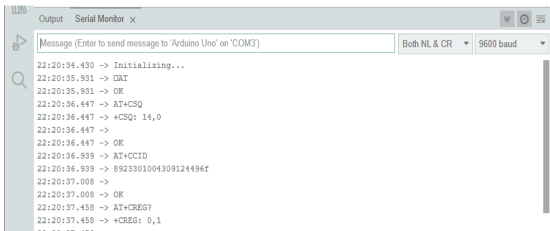
Fig. 10. GSM test result captures from Arduino sketch using AT commands
