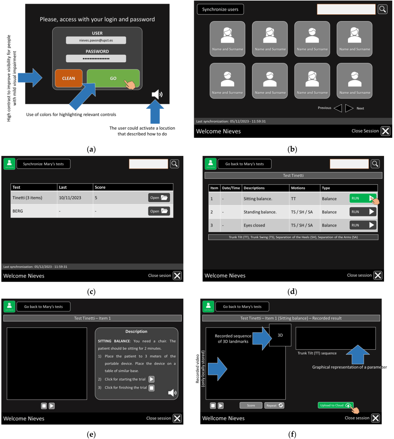
Figure 7. UI mockup for the application executed in the portable device. (a) Login screenshot; (b) List of patients (elderly people) attached to a caregiver; (c) List of tests prescribed to a patient; (d) List of items included in a selected test; (e) Screenshot of a selected item ready to be executed; (f) Results of the executed item.
