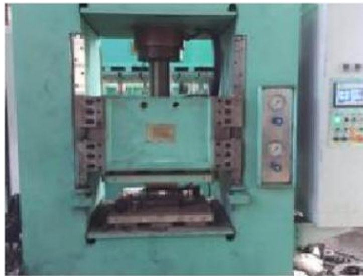
Fig. 5. Metal bipolar plate stamping machine
