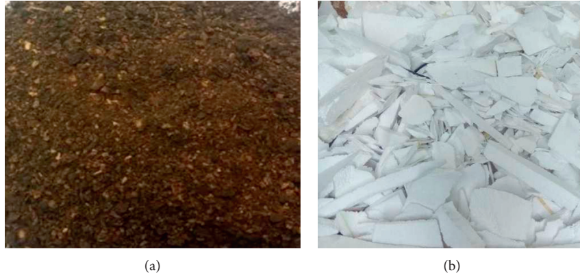
FIGURE 1: Feedstock material for co-pyrolysis oil. (a) Neem de oiled cake. (b) Waste polystyrene.
