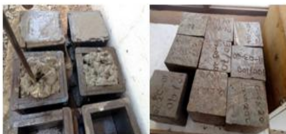
Fig. 6. Samples of cubes being moulded
