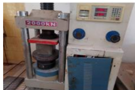
Fig. 8. A cube being crushed in a compression machine
