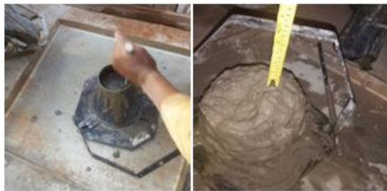
Fig. 5. Slump test being conducted on fresh concrete
