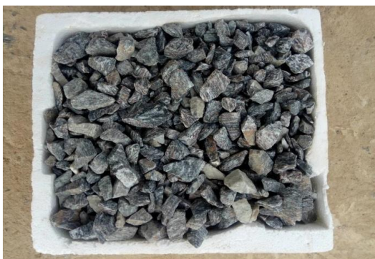
Fig. 2. Sample of coarse granite aggregate used
