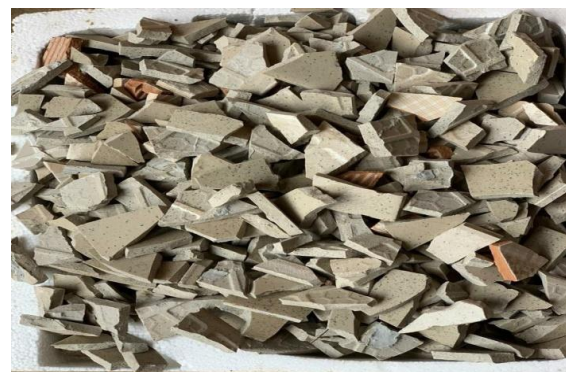
Fig. 3. Sample of ceramic waste aggregate used
