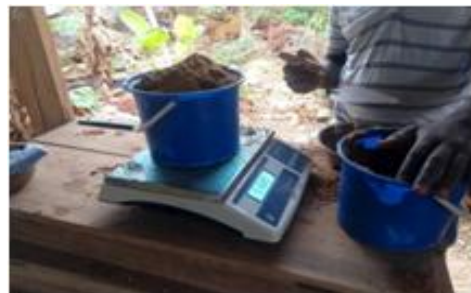
Fig. 4. Batching process of the constituent materials
