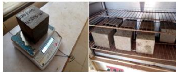
Fig. 7. Weighing and oven-drying of cube specimens
