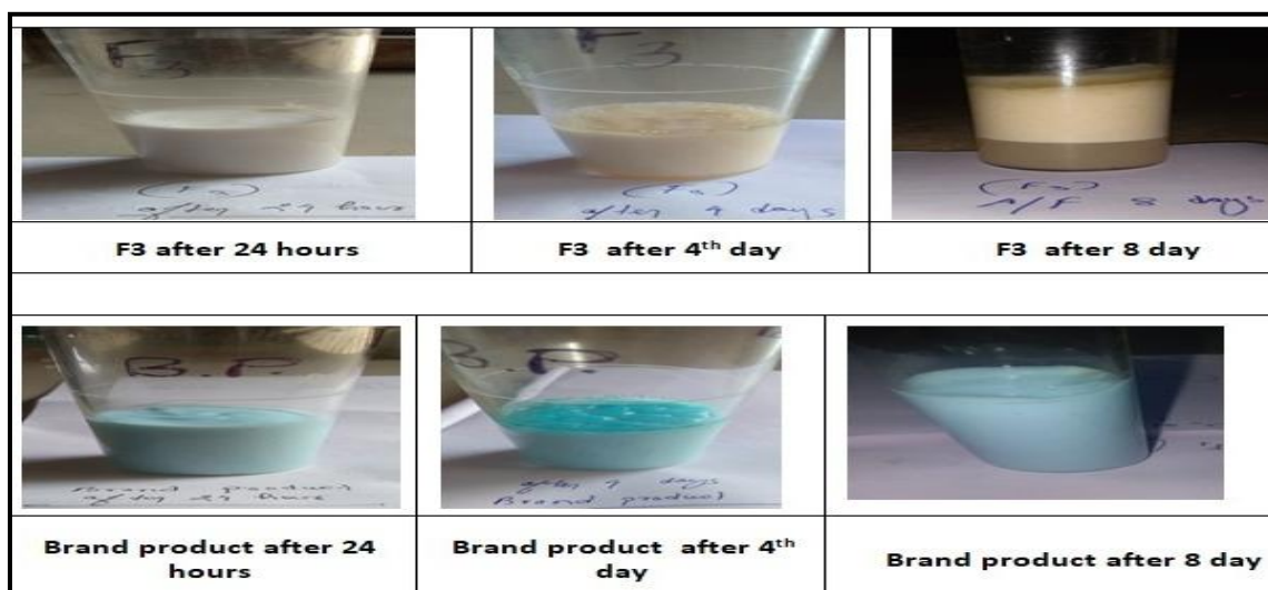
Fig. 8. Stability study of formulation (under elevated temperature exposure (55°C))
