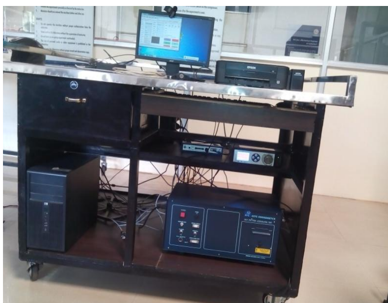
Fig. 2 (a). The pollution testing exhaust gas analyzer apparatus
