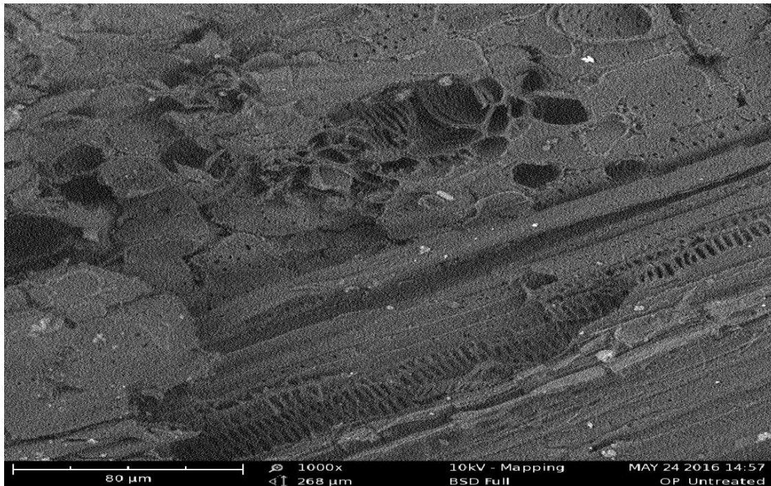
Fig. 2b. SEM of pretreated oil palm frond
