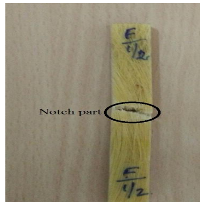
Fig. 7. Flexural test specimen after fracture
