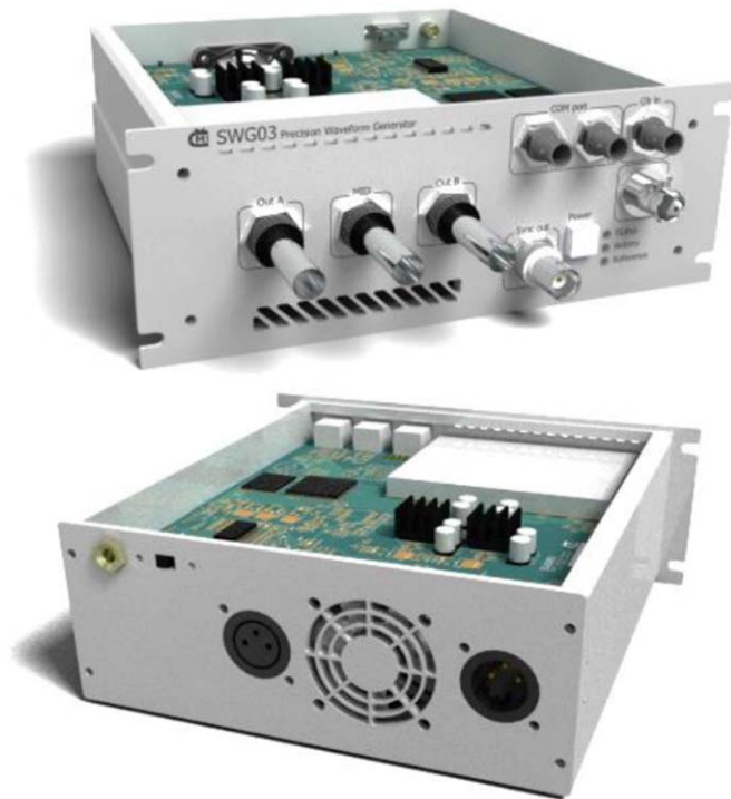
Figure 4. View of a SWG generator module without the top cover. Upper: front view—channel A and B outputs (left), communication and clock optical fiber cable connectors (right top), external voltage reference input (center right), status LEDs (bottom right). Lower: rear view—power supply output for custom electronics (middle), fan outlet, charger input (right).
