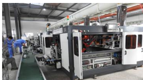
Fig. 1. The automatic bacillus bagging machine
