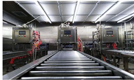
Fig. 3. The automatic bacillus bagging machine
