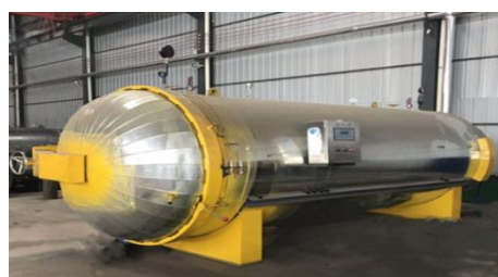
Fig. 2. The Double-door autoclave steam sterilizer
