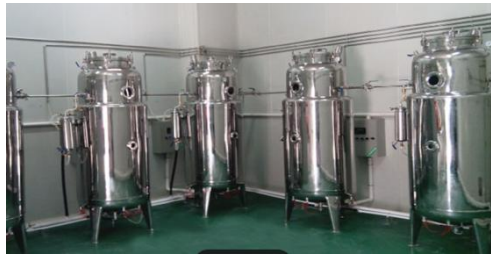
Fig. 5. The bit sterilization fermenter
