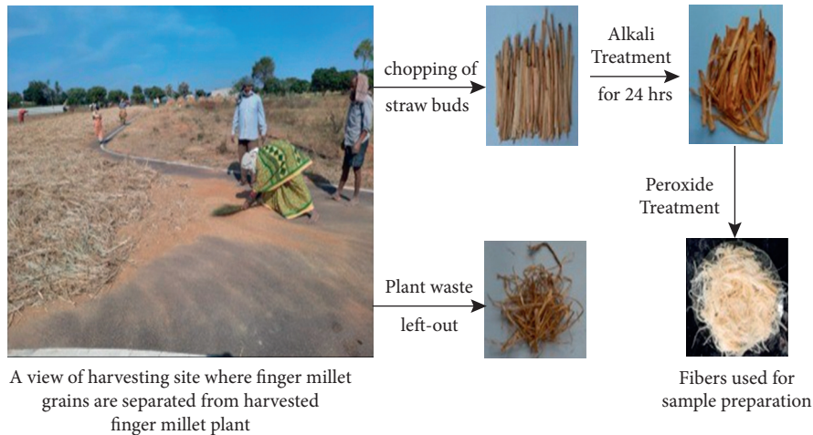
FIGURE 1: Fiber extraction from finger millet straws at Bandipalya.
