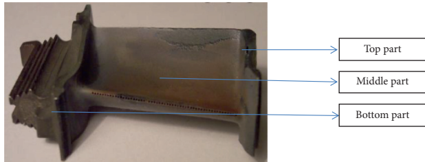
FIGURE 42: The 3-part division of the turbine blade.
