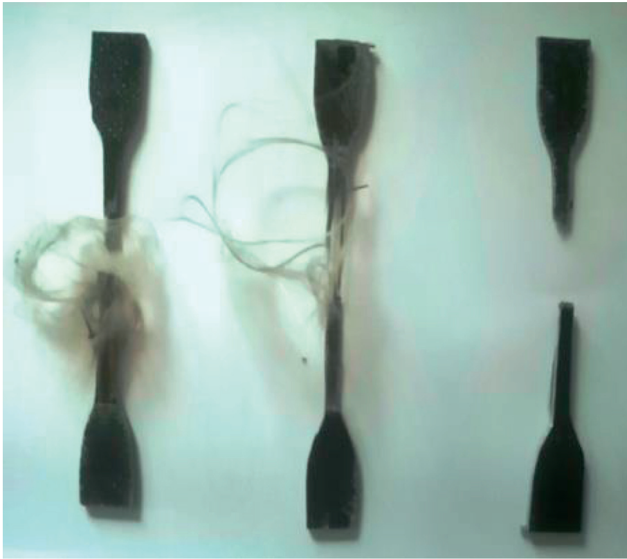
FIGURE 6: Representations of tensile tested samples for (a) laminate L1; (b) laminate L2; (c) laminate L3.
