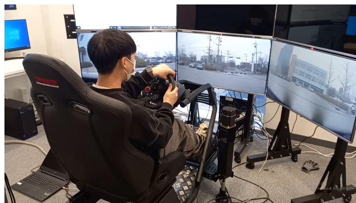
Figure 2. Example of the teleoperation which controls teleoperated vehicle using 5G/LTE network. Camera scenes are transmitted after compression and sent to the control center within about 43 ms on average.
