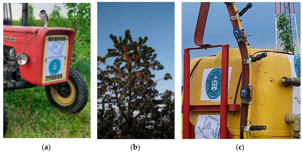
Figure 9. Tractor equipment for spraying: (a) side camera placed on the hood for classifying trees and controlling the sprayer, (b) example image collected by the side camera, (c) orchard sprayer with an attachment equipped with solenoid valves controlling the inlet into spray nozzles.
