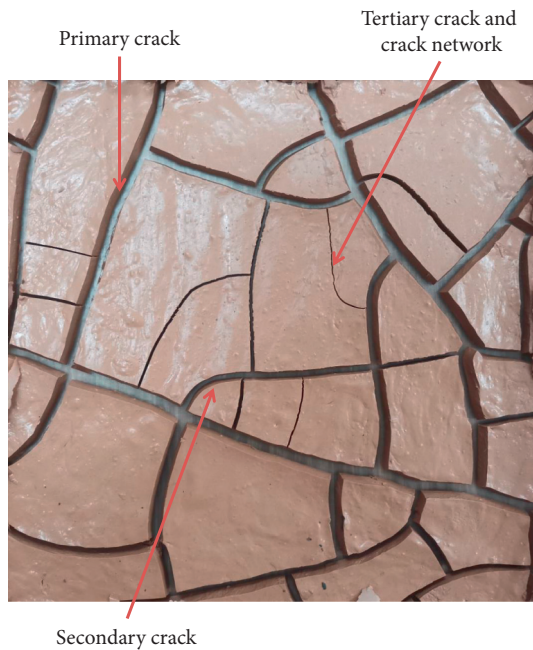
FIGURE 4: Tertiary crack development of sample.
