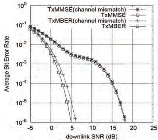
**Figure 4.** Average BER performance of the downlink Tx beamforming schemes with both the MMSE and MBER designs for the TDD-SDMA induced MIMO system which consists of a four-antenna BS to support four single-antenna BPSK MTs, when the downlink and uplink channels mismatch.
